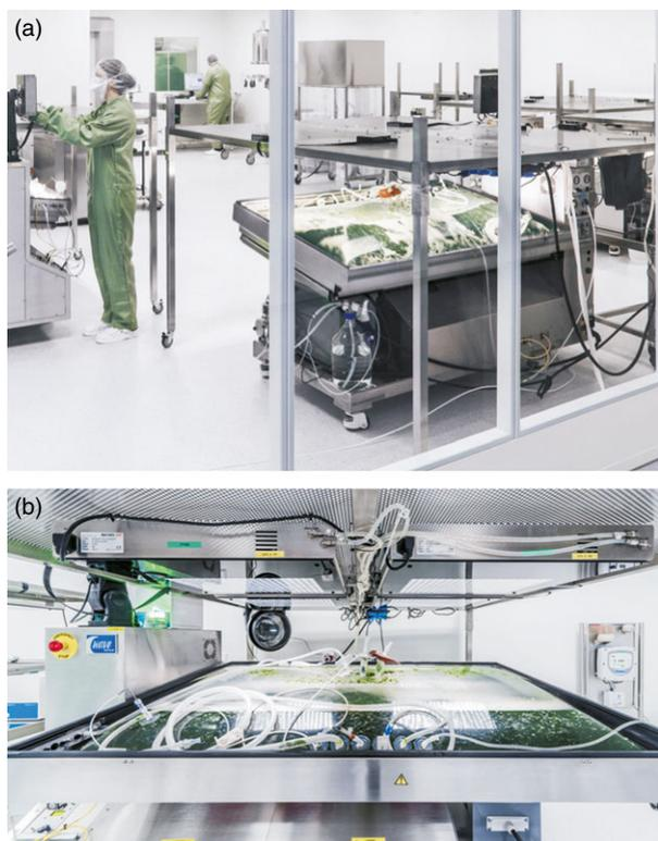
**Figure 1** Industrial-scale, GMP-compliant disposable wave reactors for the production of biopharmaceuticals expressed in the moss *Physcomitrella patens*. (a) A room equipped with several wave bioreactors. (b) A detailed view on a wave bioreactor and its illumination system. Images are courtesy of Greenovation Biotech GmbH.
