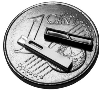
Fig. 2 Photograph picture of the two presented agent release cartridges. The lower tool is the single channel agent release cartridge, the upper one the double channel agent release cartridge. The diameter of the coin is d=16.25 \text{ mm}
